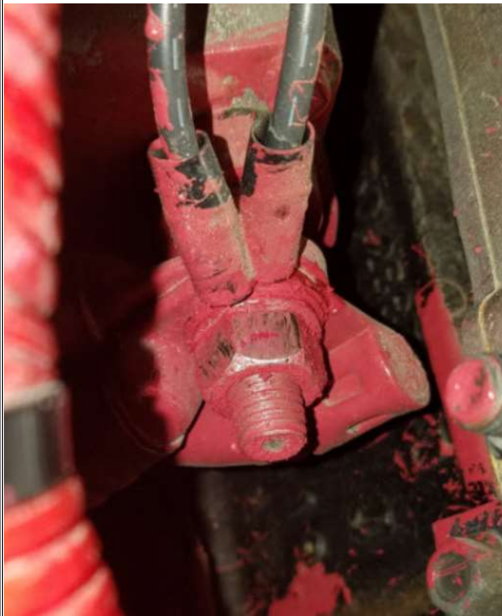
Figure #2: Coating Thinned/Removed via Wire Brush/Scraper
