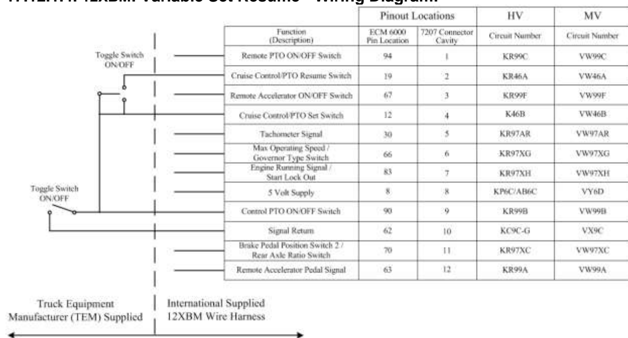
Wiring Diagram for 12XBM Variable Set Resume Speed Function (Severe & Medium Vocational Series)
