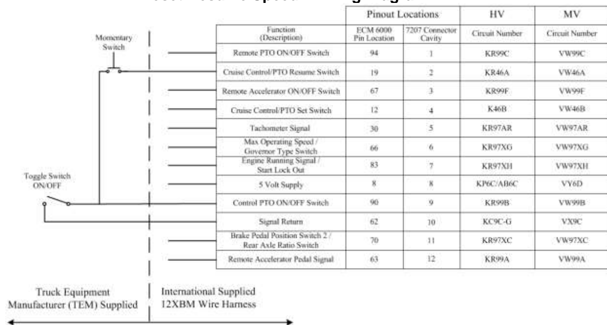
Wiring Diagram for 12XBM Preset Resume Speed Function (Severe & Medium Vocational Series)
